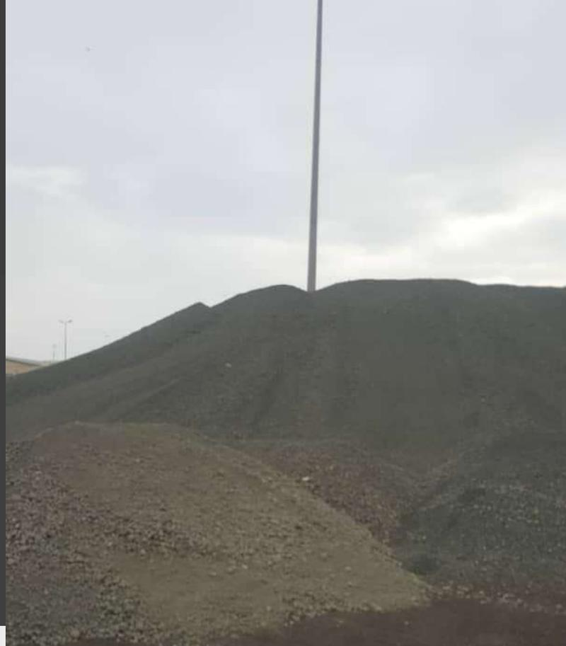
Clinker is a nodular material produced in the kilning stage during the production of cement and is used as the binder in many cement products. The lumps or nodules of clinker are usually of diameter 3-25 mm and dark grey in color.
