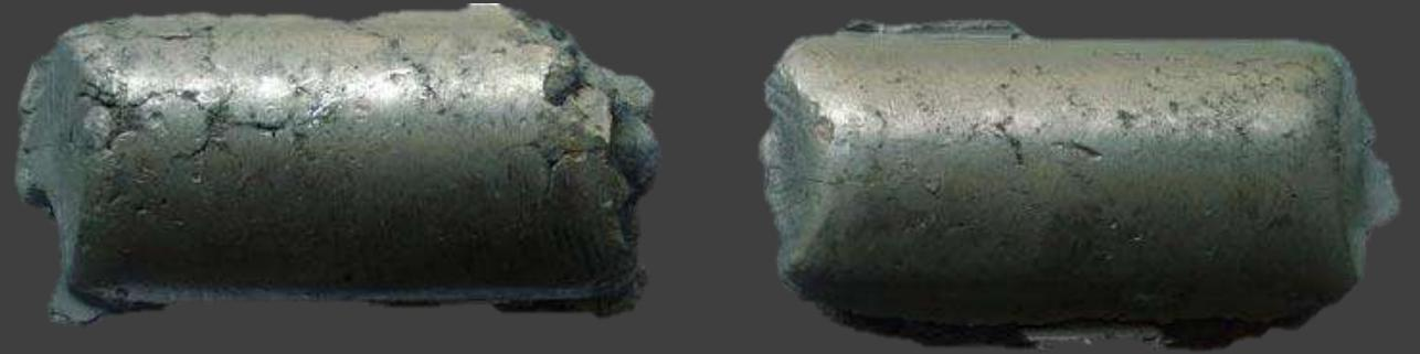
**HBI** stands for hot briquetted iron – porous sponge iron, pressed into briquettes. **HBI** is created by reducing the iron ore with natural gas. **HBI** can be **used as** a pre-material in blast furnaces or electric arc furnaces.
